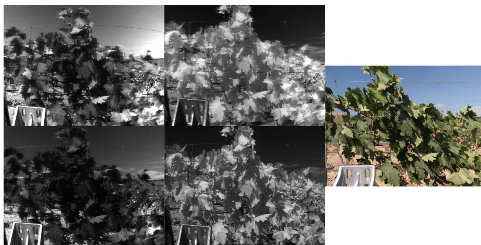
Figure 13. On-the-go acquisition of a Sequoia's measurement. Four spectral channels and one RGB image are taken per measurement. NDVI must be computed from two of these channels
