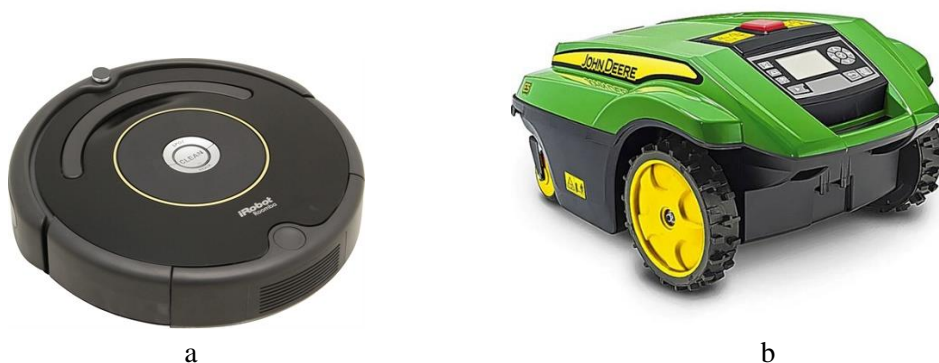
Figure 37. Service robots: a) vacuum cleaner Roomba by iRobot; b) Tango autonomous mower by John Deere
